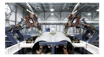
➤ F/A-18 STRUCTURAL REFURBISHMENT PROGRAMS Installation of more powerful and robust structural components to extend the platform's service life [from 5000 to 6000 flight hours].
