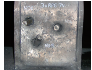
Ballistic verification – Module after live firing – 3 hits from RPG
