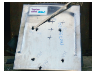
Ballistic verification – Ballistic testing against medium caliber APFSDS-T – High multi-hit performance
