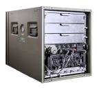
Transport container: 12 RU/610 mm deep 3 × 19" drawer every 2 RU Weight: approx. 63 kg The TAN gateway GC is the central communication point of the overall system. It includes the gateway for routing voice and IP data, as well as the communication control system.
